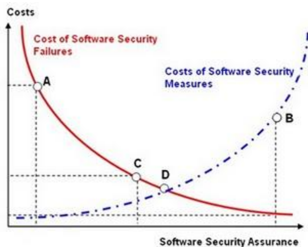
Figure 1: Cost of Investment in software security measures against failure costs due to incidents that exploit software vulnerabilities. At the point (A) to the costs due to software security failures exceed of several order of magnitude the expenditure in countermeasures and the assurance on the security of the software is very low, on the contrary in (B) the costs of security measures outweigh the costs due to the software failures, the software can be considered very secure but too much money is spent for software security assurance. In point (C) the cost of losses is nearly two times larger costs of security measures while in point (D) the costs due to incidents is equal to the cost of the security measures. The optimal value for spending of security measures is the one that minimizes both the cost of incidents and security measures and maximizes the benefit or the security of the software.
